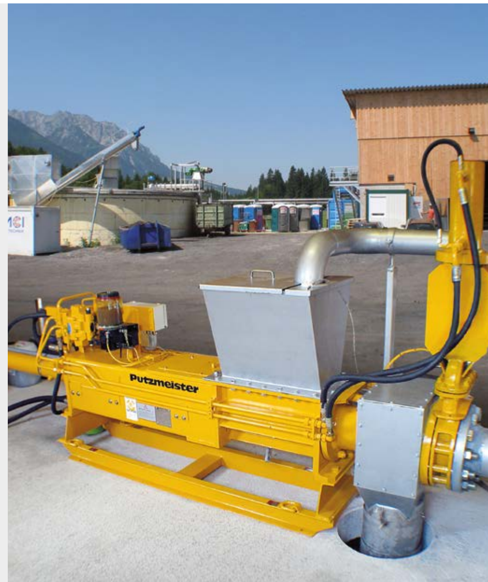
An EKO 1060 PP in a biomethanisation plant (Kössen, Austria) for unwrapping and transporting foods past expiry date
