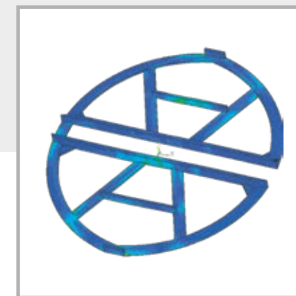
Finite element analysis for the sliding frame
