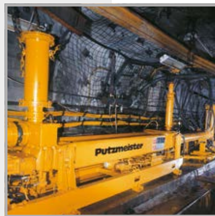
HBL slurry pumping system. Before: 43 centrifugal pumps – Now: Only two HSP 3080 solids pumps.
